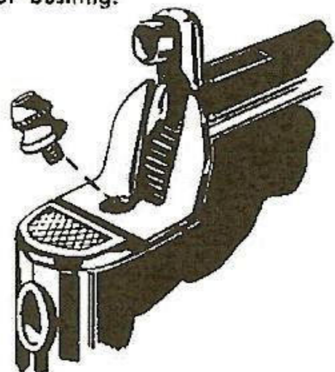
C. Unscrew chimney (Wick Holder) MA-805 with pliers and remove.
