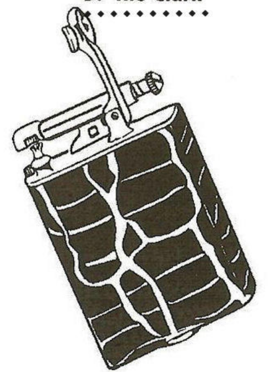
This lighter is typical of a number of thumb wheel roller type lighters all of which are constructed in the same manner and operate the same way. Parts, however, are not interchangeable.
